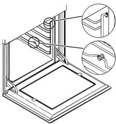
The shelf support can then be hinged upwards and lifted from the mounting holes in the upper corners of the oven prior to removal. To re-fit the shelf supports, reverse the procedure ensuring that the clip device engages firmly on the lowest runner.
